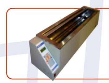
The Ductility Testing Machine is used to determine the ductility of bituminous materials in a briquette mould by measuring the breaking elongation at a constant speed. The Internal tank is made of stainless steel. The bath is fitted with an immersion heater in order to obtain (in normal conditions), the test temperature.
