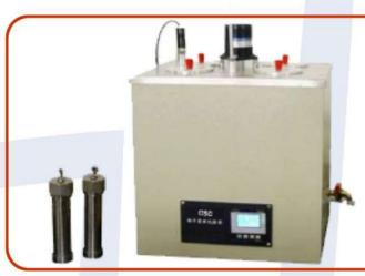
The instrument is designed and made for Detection of Copper Corrosion from Petroleum Products by the Copper Strip Tarnish Test". It is suitable to determine corrosiveness of aviation gasoline, jet fuels, vehicle gasoline, natural gasoline, hydrocarbon with Reid vapor pressure, solvent oil, diesel oil, distillate oil, lubricating oil and other petroleum products, to copper.
