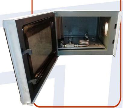
Capillary Tube Viscometer (CTV-S10)
