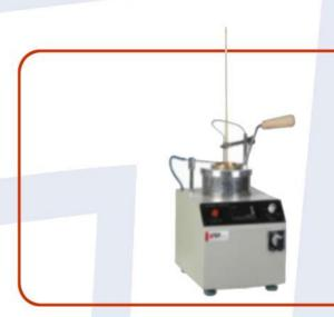
This device is used to determine the flash point value of petroleum products. It is widely used in railway, aviation, electric power, oil industry and scientific research departments, etc.
