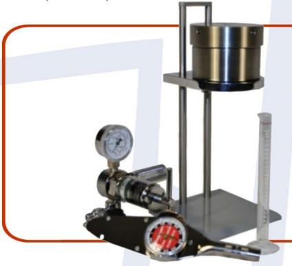
This apparatus measures the stuck tendency coefficient of a drilling fluid. The probability of the occurrence of stuck pipe situation by a drilling fluid, and also, the performance of an additive to stuck solution could be measured by this setup.
