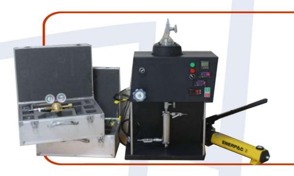
This apparatus measures drilling fluid and cement filtration at HPHT condition. Also, it is designed to be capable to conduct permeability plugging test at reservoir condition. Hence, this apparatus could provide accurate simulation and measurement of down-hole static filtration.
