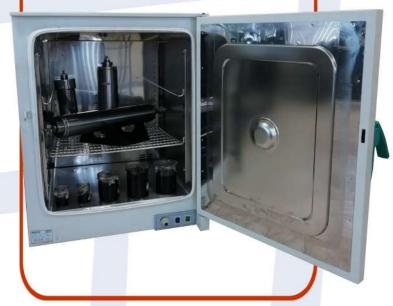
The sand pack core flooding is a vessel filled with sand and dedicated to evaluate and optimize oil recovery for different injection protocols and fluids e. g. miscible and immiscible injection, surfactant injection, polymer injection and etc.
