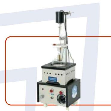
This device is designed and manufactured under GB Determination of Aniline Point in Petroleum Products for testing aniline point of dark petroleum products.
