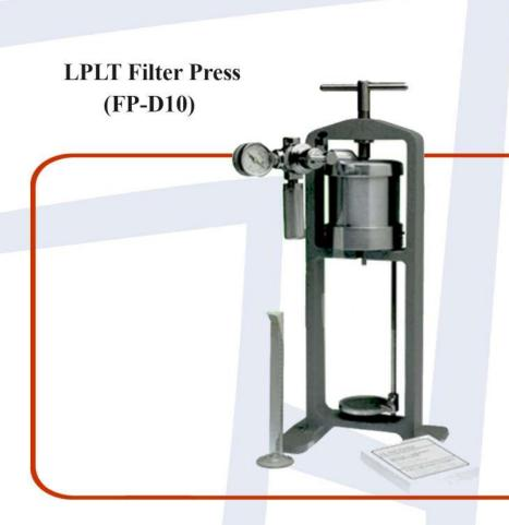
This apparatus measures drilling fluid and cement filtration at ambient condition based on API procedure. It is also applicable to check the wall-building (filter cake) properties of drilling mud and cement slurries using a filter paper.
