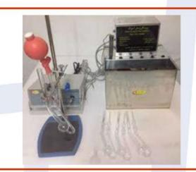
Ostwald viscometer, also known as U-tube viscometer or capillary viscometer is a device used to measure the viscosity of the liquid with a known density.
