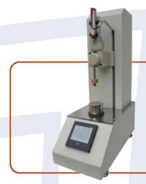
This instrument is used to determine the penetration of pavement petroleum asphalt, modified asphalt, liquid petroleum asphalt and emulsified asphalt. It is also suitable to test solid particle, powder, colloid and raw-food materials such as cheese, glycine, butter, cream and leavening. It can be widely used in food industry, highway engineering and other industrial fields.
