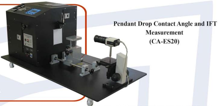
IFT as the indication of energy at the interface of two immiscible fluids; is a vital parameter for any EOR process. The EOR agents such as surfactants, alkaline and polymers tend to reduce the IFT between oil and water to decrease capillary forces and recovering more residual oil.
