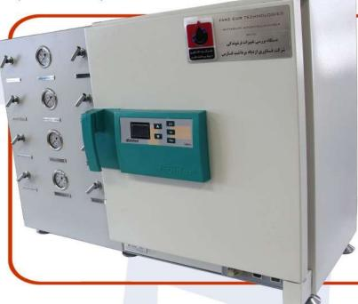
Wettability alteration chamber is designed for the purpose of core wettability restoration prior to SCAL studies. Wettability changes are obtained by subjecting the core to reservoir conditions of temperature and pressure for weeks. At this stage, a wettability transition may occur in the oil-invaded pores depending on the stability of the thin water films, located between the pore walls and the oil.
