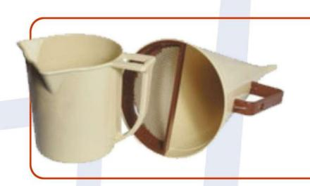
This apparatus simply measures the viscosity of drilling fluid and cement slurries. Funnel viscosity is reported as the time (in seconds) which is required for one quart of sample to pass the funnel. Marsh funnel is made up of rugged plastic resists to deformation caused by temperature change. Also, the measuring cup is graduated in cubic centimeters.
