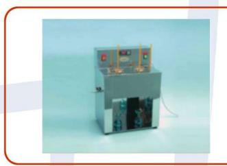
The saybolt viscometer controls the heat of the fluid and the viscosity is the time is takes the fluid to fill a container. This viscometers are most commonly used for fieldwork to measure the viscosity of oils, syrups, varnish, paints and Bitumen emulsions.
