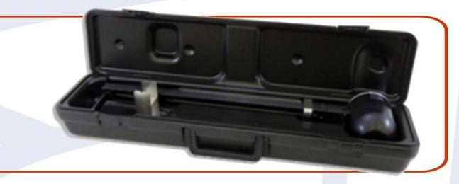
Mud balance measure the density and specific gravity of drilling fluid and cement slurries. This apparatus is designed based on API recommended practice. It is designed portable to be carried to rig in order to on-site measurement.
