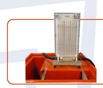
Venturi meters are flow measurement instruments which use a converging section of pipe to give an increase in the flow velocity and a corresponding pressure drop from which the flow-rate can be deduced. They have been in common use for many years, especially in the water supply industry.
