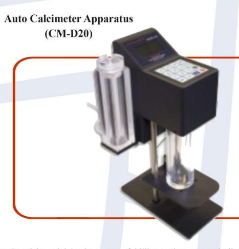
This apparatus measures the calcite and dolomite content of drilling cuttings automatically. Pressure data is transmitted to the software, and analysis is performed by the online software. Hastelloy cell resistant to hydrochloric cell is designed as reaction cell.
