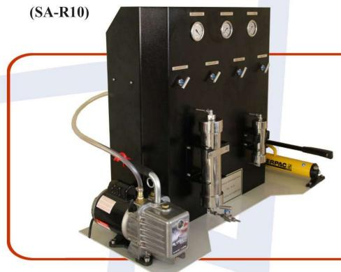
The manual saturator is used to saturate the core plug size by evacuating the air packages and inserting the pressurized fluids into the core under the pressure of maximum 300 bar. The standard apparatus includes a plug sized core cell, a vacuum pump, a hydraulic pump, a saturant vacuum tank and necessary hand operated valves and plumbing. A larger capacity cell to accommodate full size core samples is also available upon to the request.
