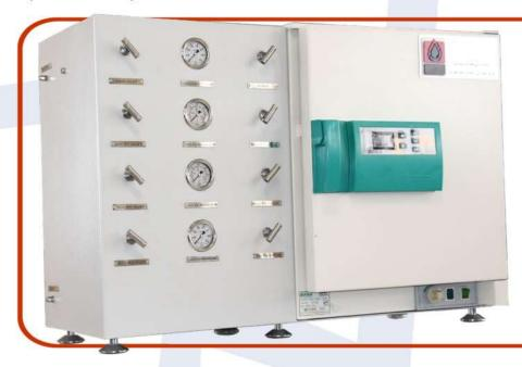
Wettability alteration chamber is designed for the purpose of core wettability restoration prior to SCAL studies. Wettability changes are obtained by subjecting the core to reservoir conditions of temperature and pressure for weeks. At this stage, a wettability transition may occur in the oil-invaded pores depending on the stability of the thin water film, located between the pore walls and the oil.
