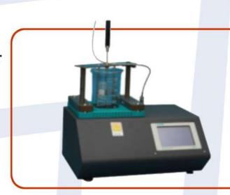
The instrument is designed and made as per the national standard Test Method for Softening Point of Asphalt. It is suitable to determine the softening point of asphalt, tar, liquid asphalt and other types of asphalt. It is the best choice of asphalt manufacturers, highway and bridge construction companies, college and universities, and research and development departments.
