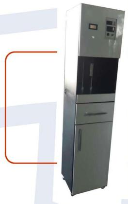
VG meter measures the direct-indicating viscosity and the gel strength of drilling fluid. It is a rotational cylinder and bob rheometer. This instrument has 6 variable speeds. When the outer cylinder is full of drilling fluid, the inner cylinder rotates at a specific velocity. So, the torque which is exerted to the inner cylinder is measured accurately. Viscosity is calculated based on the torque measurement.
