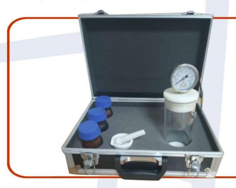
This apparatus measures the calcium carbonate (calcite) and magnesium carbonate (dolomite) content of drilling cuttings. The test is based on the reaction between calcite and dolomite with hydrochloric acid and consequent carbon dioxide emission. Formation of carbon dioxide increases the cell pressure which is measured by accurate pressure gauge.
