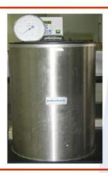
The REID Vapor Pressure Measuring Device is an automated Reid Vapor pressure instrument in full compliance with standards. These methods are for the determination of vapor pressure of gasoline, volatile crude oil, and other volatile petroleum products. The Reid method is particularly suitable for determination of vapor pressure of crude oil for transportation, storage and general handling purposes.
