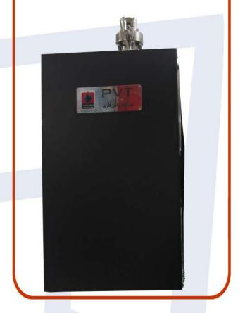
The PVT system is designed to study phase behavior of hydrocarbon fluids at reservoir conditions of pressure and temperature. It can be used to perform PVT tests on black oil, volatileoil, etc. Homogeneous sample heating is provided by a controlled temperature jacket.
