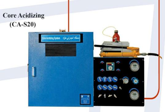
The core acidizing system is designed in a way that it is possible to inject an acid solution into a rock sample at reservoir conditions to modify the natural permibility of rock by dissolving some minerals present in the rock. Since the wetted material is hastelloy, it is possible to not only investigate the efficiency of different HCl-HF formulations to attack plugging minerals, but also to study the effects of flow rate and temperature on core samples permeability.
