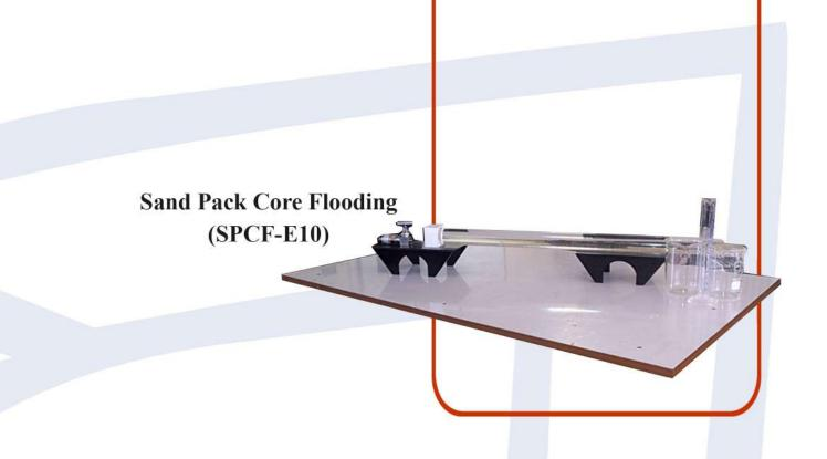
The sand pack core flooding is a vessel filled with sand and dedicated to evaluate and optimize oil recovery for different injection protocols and fluids e. g. miscible and immiscible injection, surfactant injection, polymer injection and etc.
